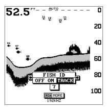
Remember, the Fish ID feature can't be used when the unit is in the manual mode. If you turn the Fish ID feature on when the unit is in manual, the microcomputer will turn the automatic feature on. If you turn automatic off when the Fish ID feature is on, the Fish ID feature will be turned off also.
